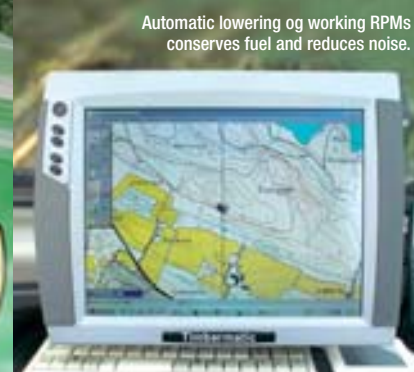
Eco III system guides the operator to more economical driving habits.
