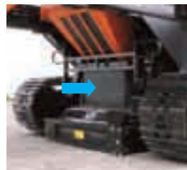
2 Opening at conveyor tail
