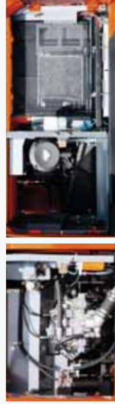
Grouped remote filters and inspection points
