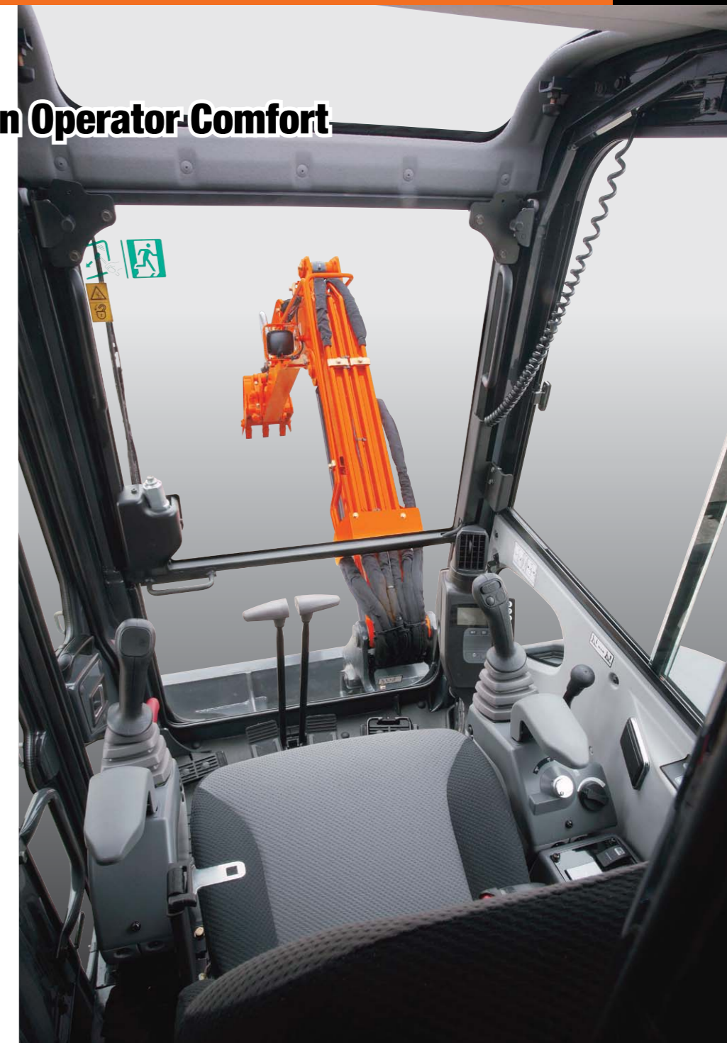
Shown is a cab specification, including options such as multi-function levers.
