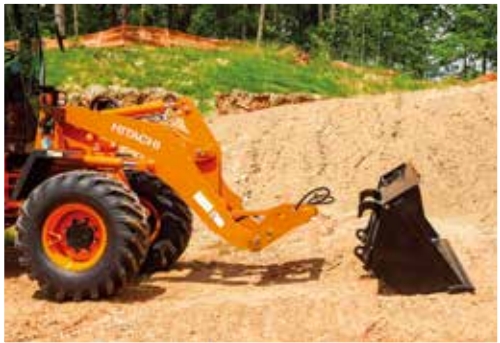
Optional pin-on type Quick Coupler allows seamless transition (mechanical for ZW30-5B / ZW40-5B and hydraulic for ZW80-5B).
