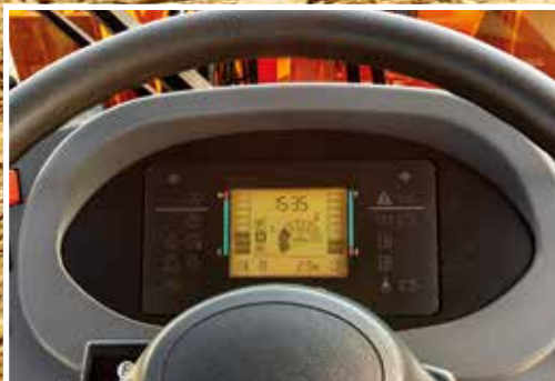
Easy to read monitor provides operating data at a glance (ZW40-5B). *ZW30-5B: Analog monitor.
