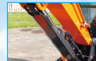
Boom cylinder guard The cylinder guard has a strong inverted V-shaped structure.
