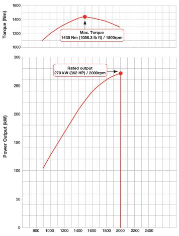
Engine Speed (rpm)
