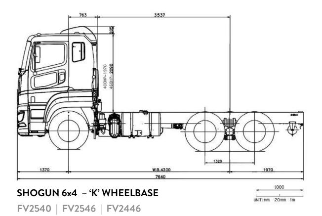
Scale = 1:50 (20mm = 1 metre). This scale is accurate when used on the original spec sheet, be aware that enlarging these illustrations can alter the scale and cause incorrect measurements. Fuso New Zealand and its authorised dealers always recommend customers seek professional advice from independent sources before commencing any engineering activities.
