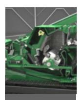
3 crush zones with optional 4th strike zone combined with an aggressive blow bar and apron design and a 4 bar variable speed rotor deliver high impact.
