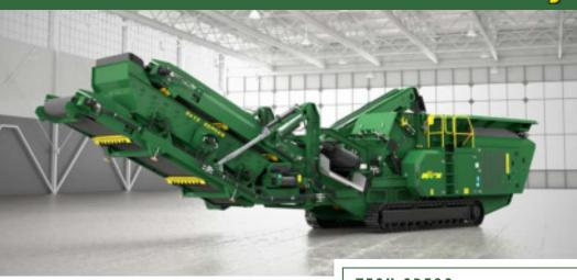
The I4C is in a class of its own, bringing the productivity of an 1125mm (44.3") impactor to a compact footprint for maximum power and maneuverability.
