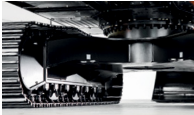
Improvements to the undercarriage have enhanced durability.
