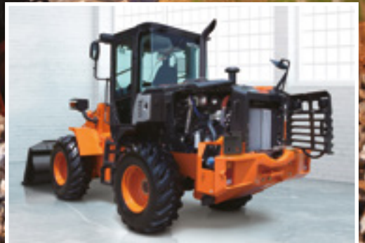
Easy access for maintenance from ground level.
