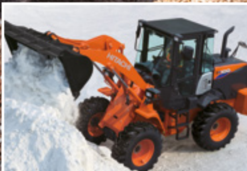
Torque proportioning differentials reduce tire slippage in wet or wintry conditions.
