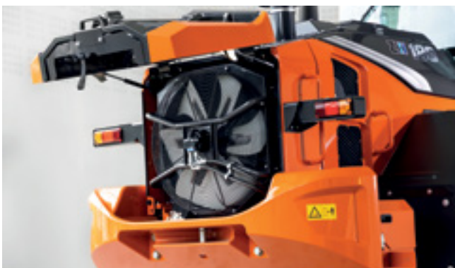
Intelligent fan operation system prevents radiators clogging.
