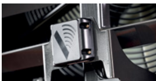
Rear obstacle detection system enhances safety on the job site. (optional NZ)
