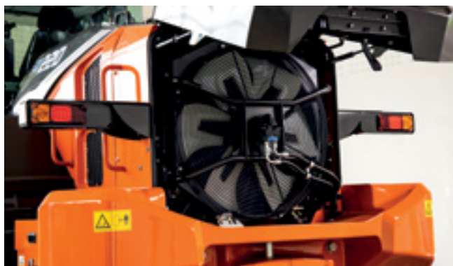
Intelligent fan operation system prevents radiators clogging.
