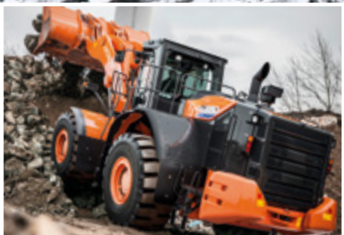
The optional belly guard provides added protection.
