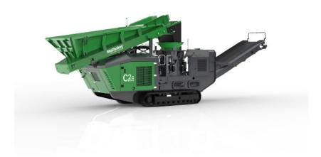
The McCloskey C2C Cone Crusher is the ideal portable secondary crushing solution for operators requiring production rates up to 300 TPH. Its unrestricted feed opening improves material feed intake and reduces the risk of blockage. The direct drive cone on the C2C has a minimum setting of 13mm (0.5") and a maximum feed of 185mm (7.28"). The variable speed of the crusher delivers the best combination of production and product shape, maximizing its efficiency in crushing.
