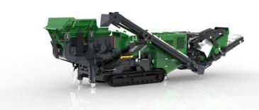
The large 1060mm (42") x 700mm (28") jaw chamber accommodates large feed sizes, contributing to higher production in material processing. The material path can be enhanced with an optional double deck 1064mm x 2215mm (41.9" x 7' 3") double deck grizzly prescreen under the hopper that, along with the variable speed pan feeder, allows for better sizing of material with a variety of mesh options.
