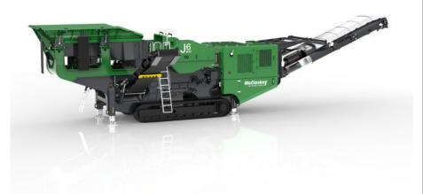
The large 1200mm (48") x 864mm (34") jaw opening accommodates large feed sizes, also contributing to higher production in material processing. The material path is enhanced with the adjustable speed 1204mm x 2360mm (47.4" x 7'-8.8") double deck grizzly prescreen under the hopper that, along with the variable speed panfeeder, allows for better sizing of material with a variety of mesh options.
