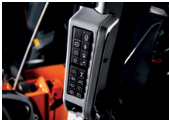
All commonly used functions can be selected at a glance using the side panel switch.
