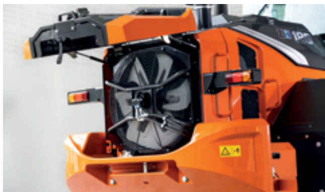
Intelligent fan operation system prevents radiators clogging.
