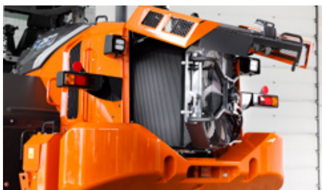
Intelligent fan operation system prevents radiators clogging.
