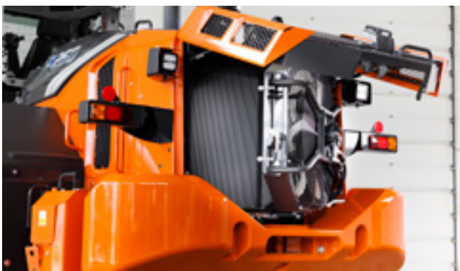
Intelligent fan operation system prevents radiators clogging.
