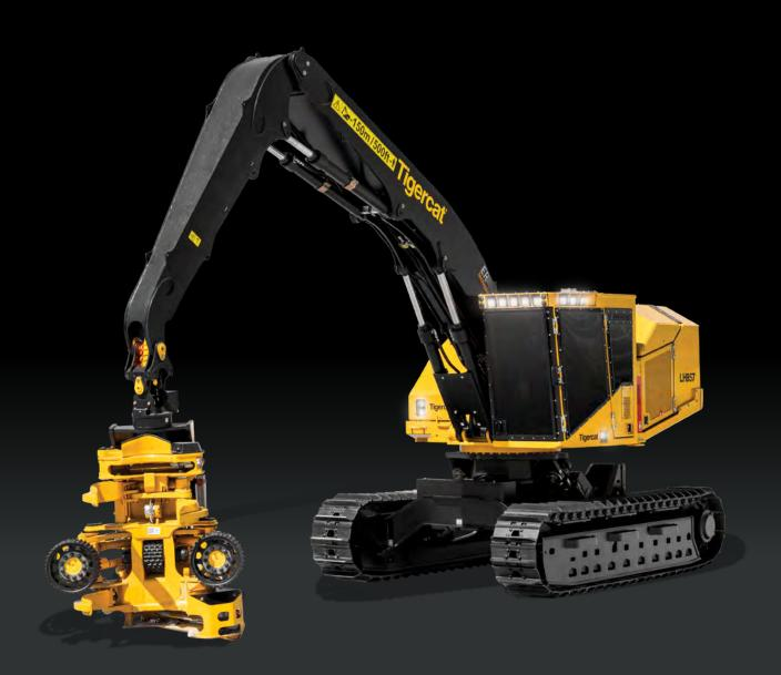
STEEP SLOPE HARVESTER WITH SLOPING TAIL FOR INCREASED LEVELING CAPABILITY.
