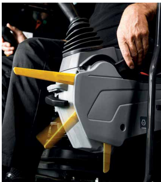
The pilot shutoff lever offers enhanced safety in the cab.
