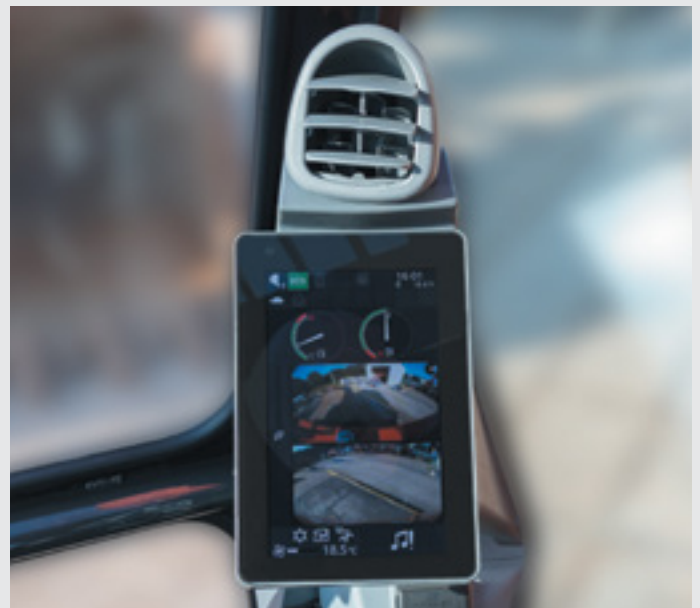
Low-reflective color 8" monitor. Easier to view and navigate. Bluetooth® and USB power supply available.
