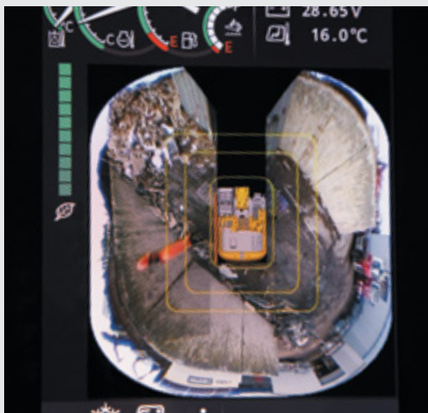
AERIAL ANGLE 270-degree bird's eye-view camera system gives exceptional visibility from the cab.
