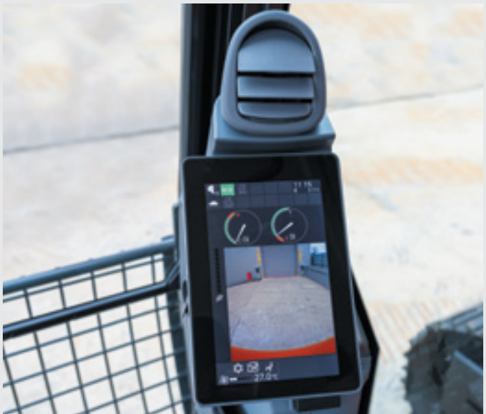
Low-reflective color 8" monitor, 42% larger display compared to ZX-5G series. Easier to view and navigate. Bluetooth® and optional USB power supply available.
